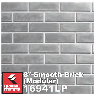
8" Smooth Brick (Modular) 16941LP 16941LP 8" Smooth Brick (Modular) Max Depth: 0.25" Brick Size: 7.625"W x 2.25"H
