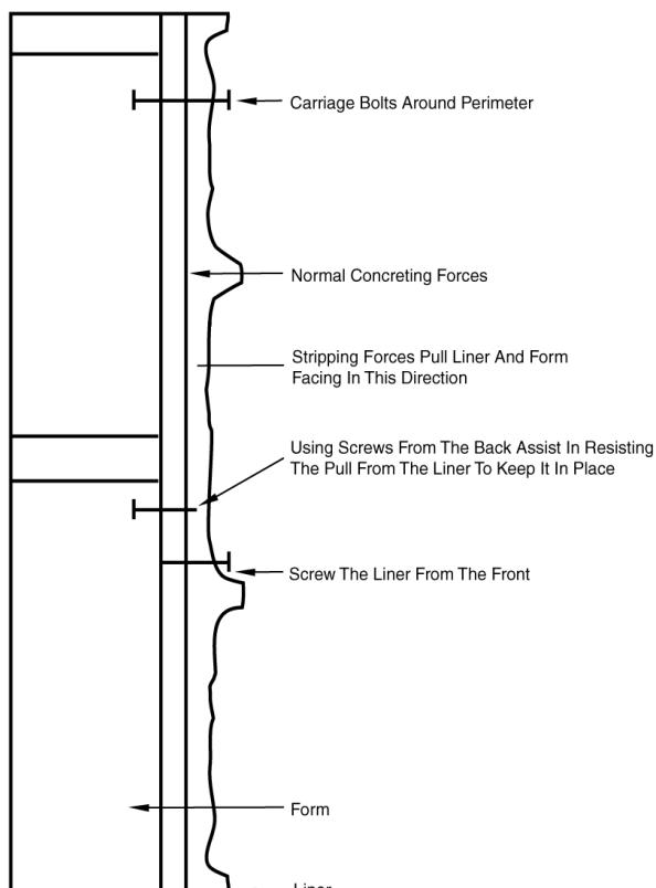
To assist in removal from the wall, adequate formliner attachment is critical. (Please refer to the illustration to the left.) Attaching the liner should occur from both the front and back sides of the form. Through the front-side, embed 1/4" carriage thru-bolts on 12" centers along all outside edges of the liner. At 18"-24" centers through the field of the liner, embed 1/4" coarse screws directly into the formliner plywood.
